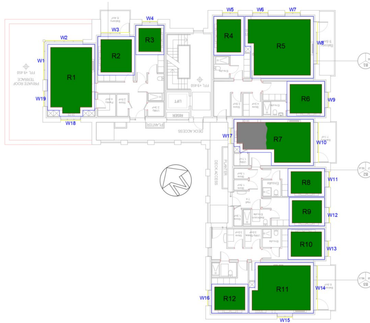
Figure 28: Apartment Block 1 Third Floor sDA Contours
