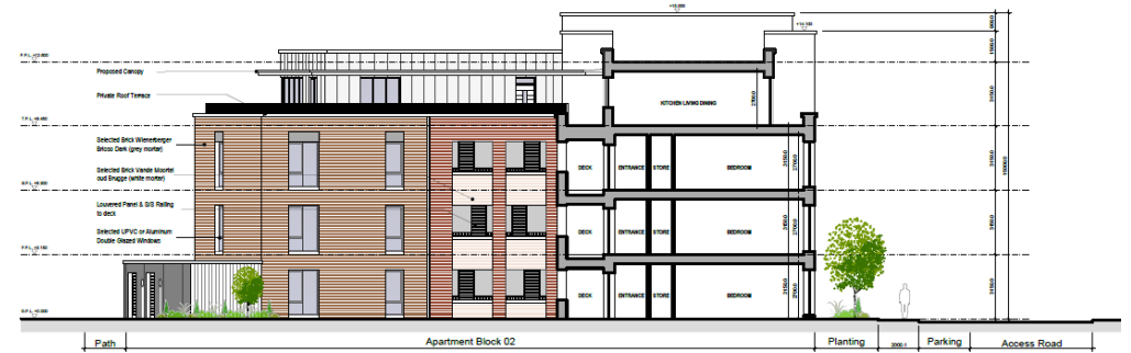
Apartment Block 02 - South East Sectional Elevation Scale 1:200
