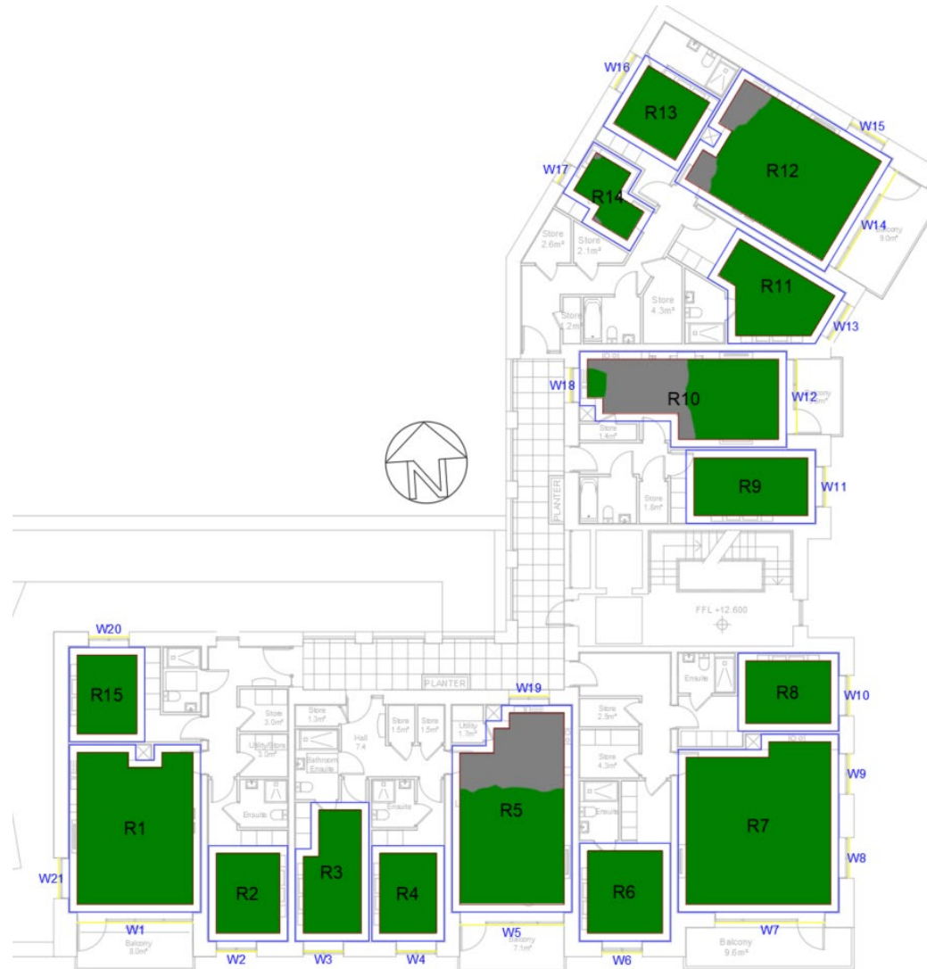
Figure 45: Apartment Block 5 Fourth Floor sDA Contours
