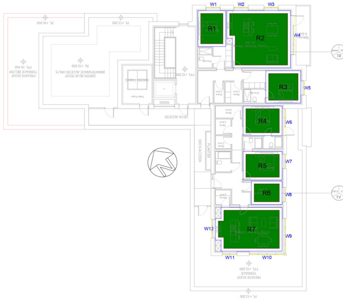
Figure 29: Apartment Block 1 Fourth Floor sDA Contours
