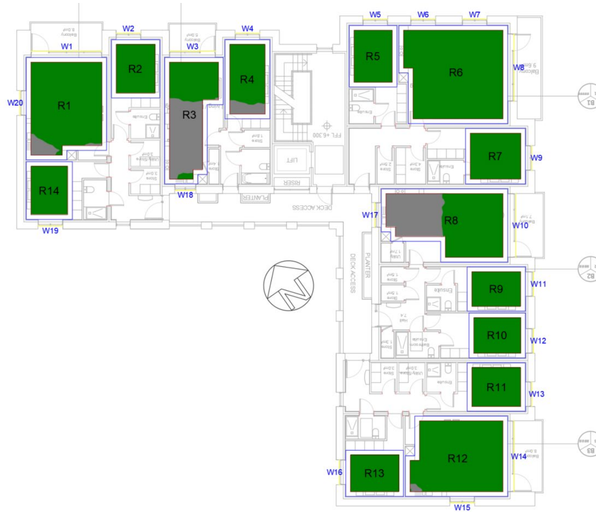
Figure 27: Apartment Block 1 Second Floor sDA Contours
