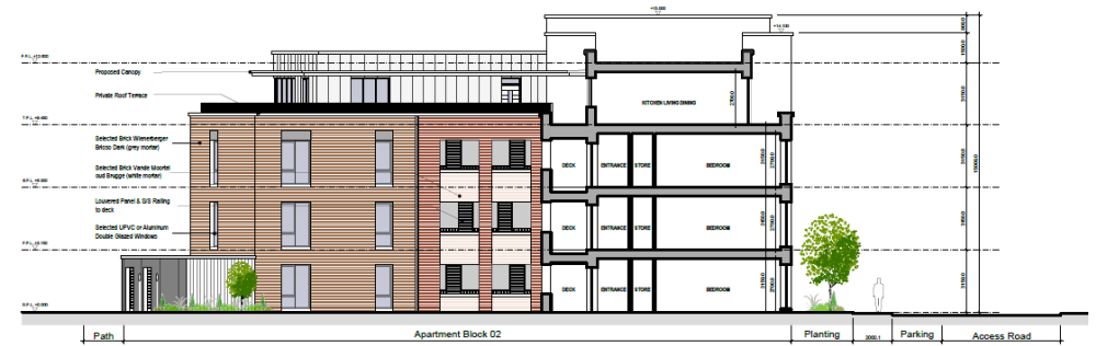
Apartment Block 02 - South East Sectional Elevation
