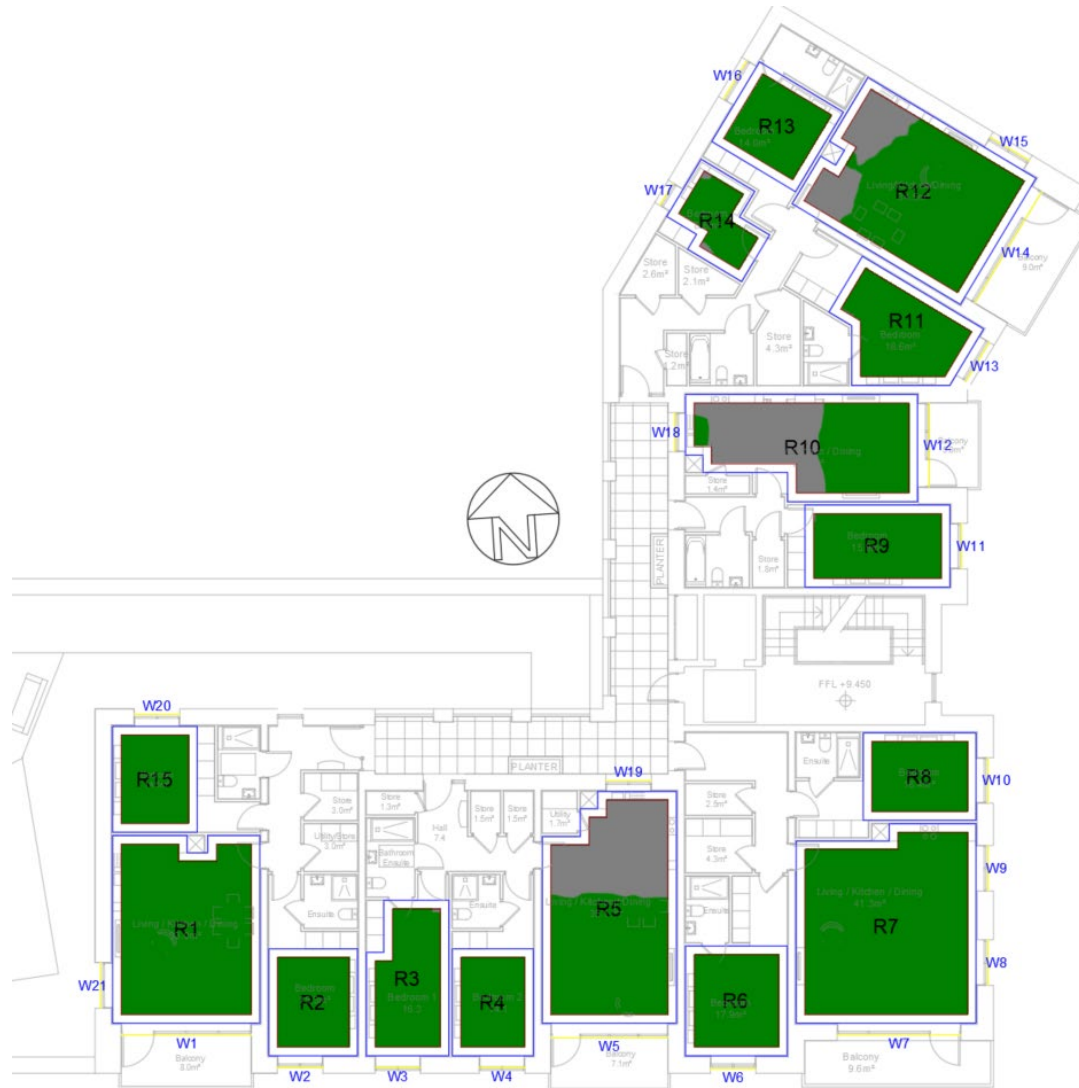
Figure 44: Apartment Block 5 Third Floor sDA Contours
