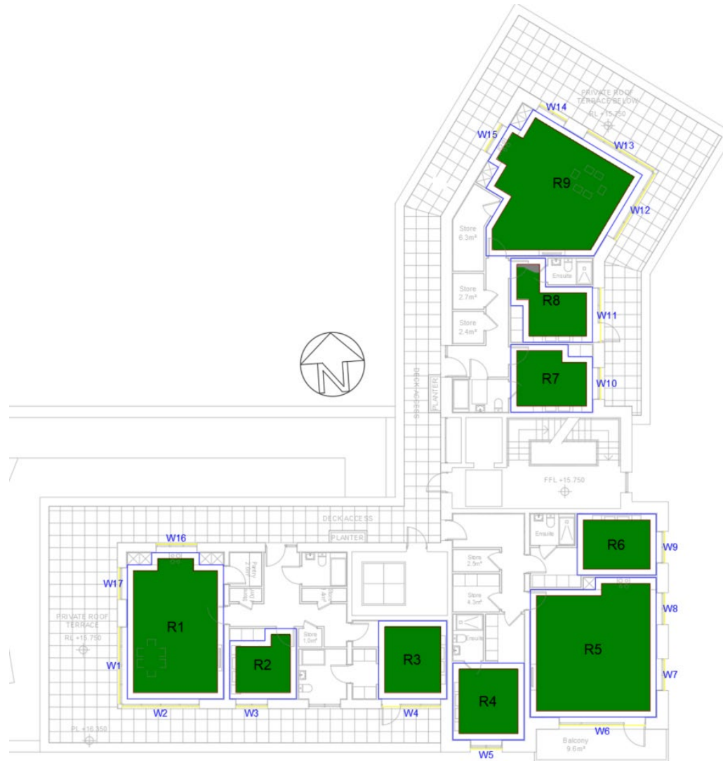
Figure 46: Apartment Block 5 Fifth Floor sDA Contours
