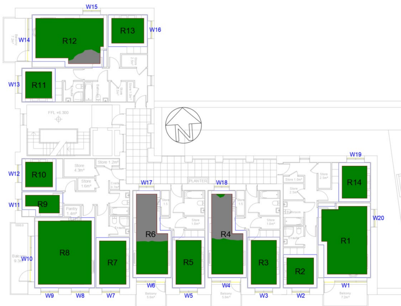
Figure 38: Apartment Block 4 Second Floor sDA Contours
