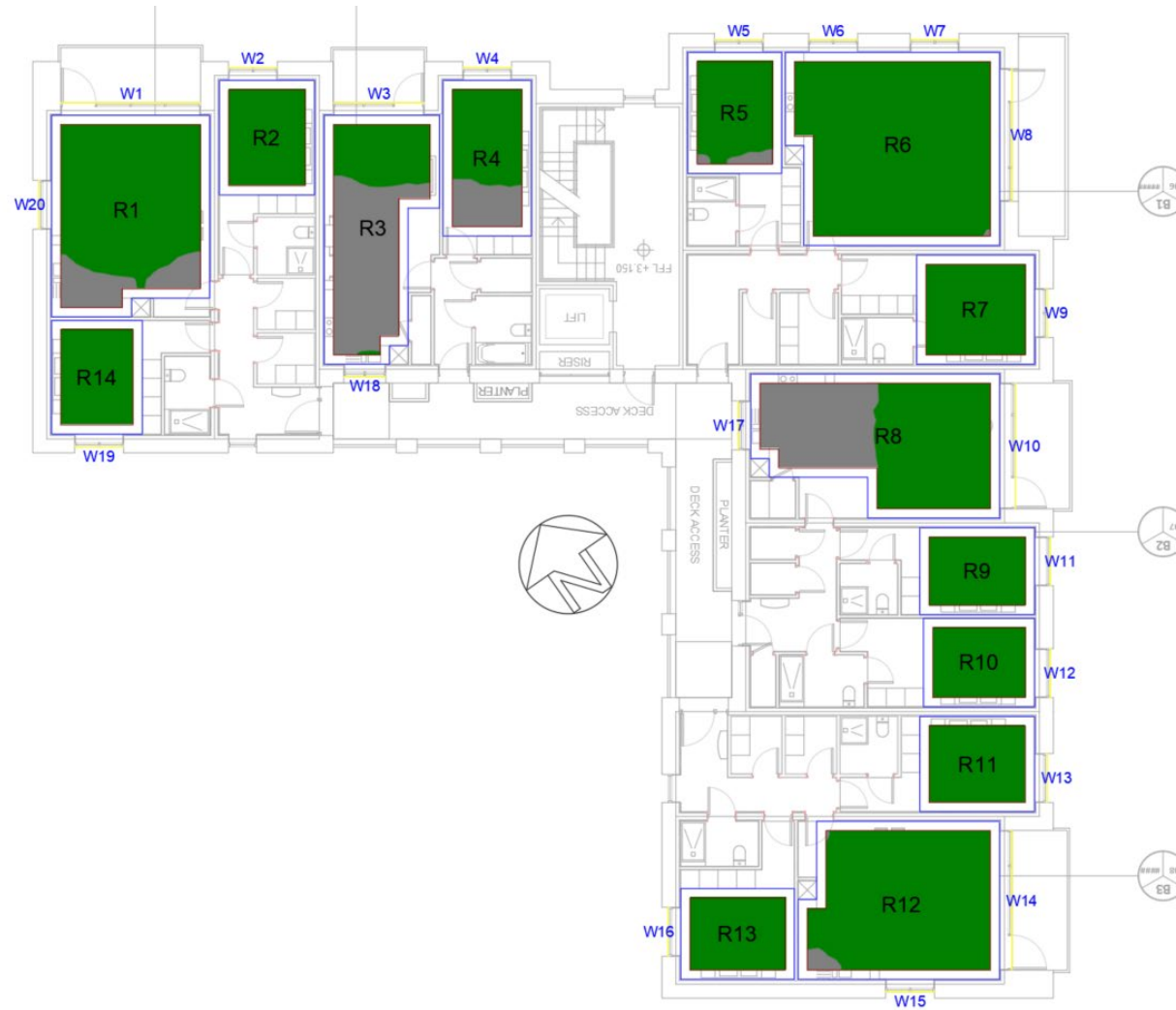
Figure 26: Apartment Block 1 First Floor sDA Contours
