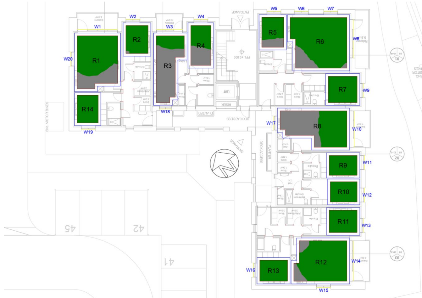
Figure 25: Apartment Block 1 Ground Floor sDA Contours
