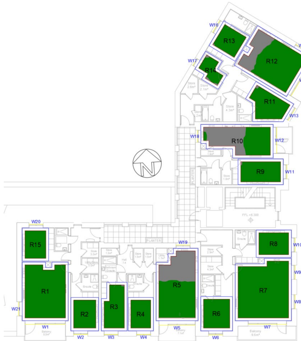
Figure 43: Apartment Block 5 Second Floor sDA Contours
